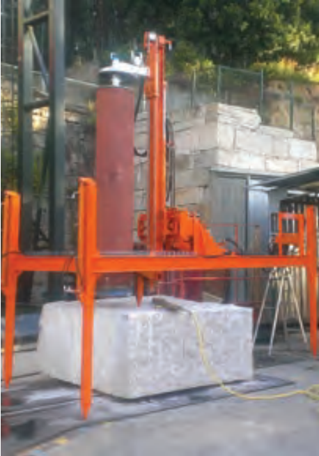
UNDERWATER DRILL FOR ROCKY SEABEDS
